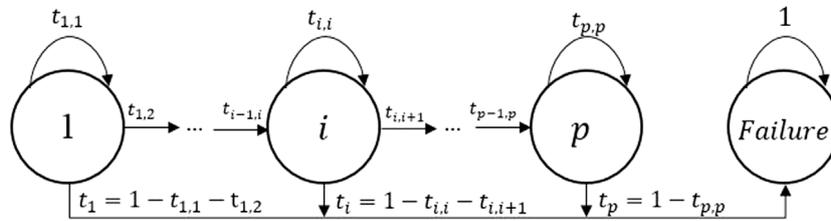
Fig. 2. Diagram of a Markov chain widely used for approximation.
