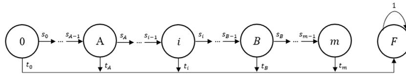
Fig. 3. Diagram of a Markov chain representing an aging process.
